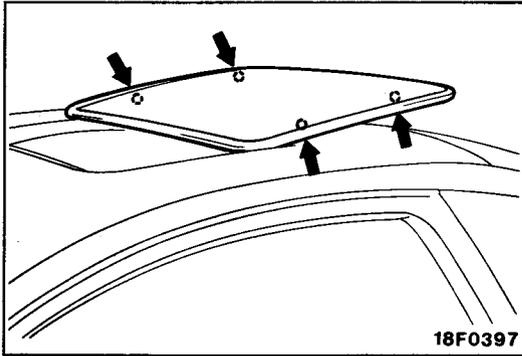
**REMOVAL SERVICE POINTS****◀A▶ ROOF LID TRIM/ROOF LID REMOVAL**
