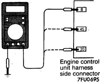
Measure the power supply voltage of the air conditioner circuit.
